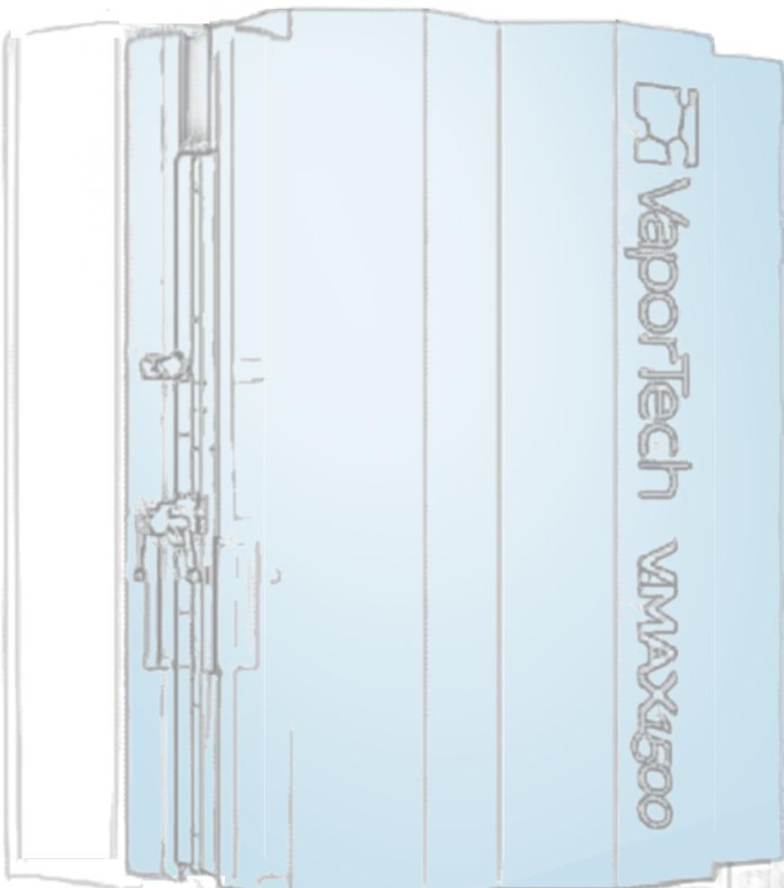
The V.MAX1500 system was designed for coatings that really perform. It offers a combination of up to 6 wall-mounted cathodic arc and/or magnetron sputtering sources for ultimate flexibility and speed. It gives you fast and flexible loading and unloading with 6 or 12 rack positions on a removable turntable. One chamber deposits PVD and DLC coatings and plasma nitriding.
